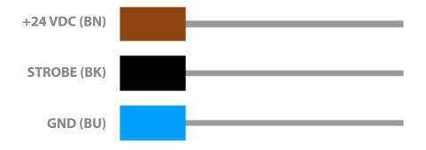
Strobe signal (black wire) between +5VDC and +24VDC. Minimum triggering current of 0.01A.
