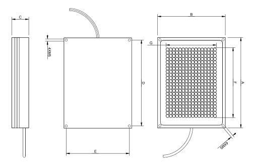
Tolerance of  $\pm 0.5$  mm applies to all of the dimensions given.
