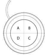
Turn on all four lighting segments by connecting all cables to a single +24 VDC supply voltage.
