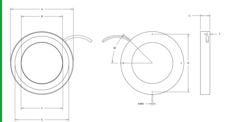
Tolerance of  $\pm 0.5$  mm applies to all of the dimensions given.
