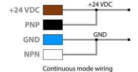
When turning on wait for at least 1 second before capturing first image in continuous mode.
