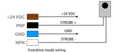
PNP voltage 5-24 VDC Min strobe current 0,01 A Max strobe frequency 1000 Hz NPN voltage below 1 VDC
