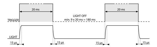
Illuminator in overdrive mode is controlled by trigger input coming from external controller or camera. Rest time between consecutive trigger inputs must be at least 9 times longer than trigger time. During rest time any additional trigger inputs will be ignored.
