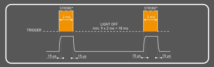
Mode If the duration of the trigger signal pulse is 5 milliseconds, the rest period between subsequent pulses must be equal to or longer than 45 milliseconds (9x5 = 45 ms).
