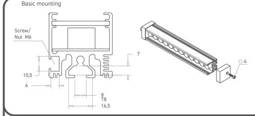
The illuminator can be rear-mounted using a T-slot and T-bolt (size 8) or side-mounted using an M6 screw/nut. It is recommended to mount it on the metal structure of the machine with maximum surface contact to reduce vibrations and improve heat dissipation.
